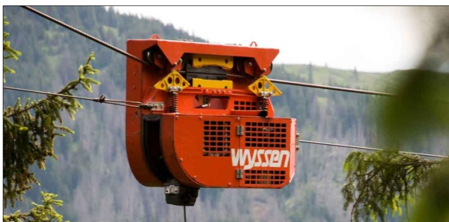
Slika 5: Samovozna kolica (( https://progresstechnik.com/en/logging/carriage )
