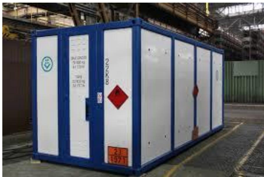
Slika 18. MEGC (Multiple element gas container) kontejner
