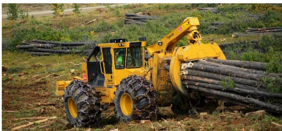
Slika 11. Grapple skidder Tigercat 630E
