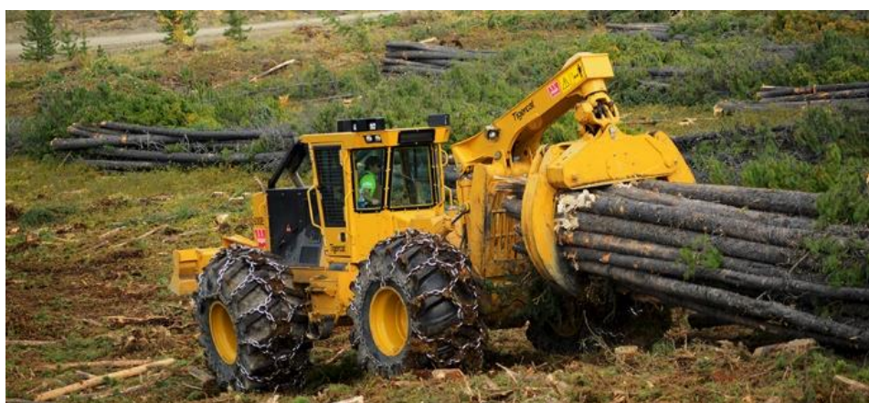
Slika 11. Grapple skidder Tigercat 630E
