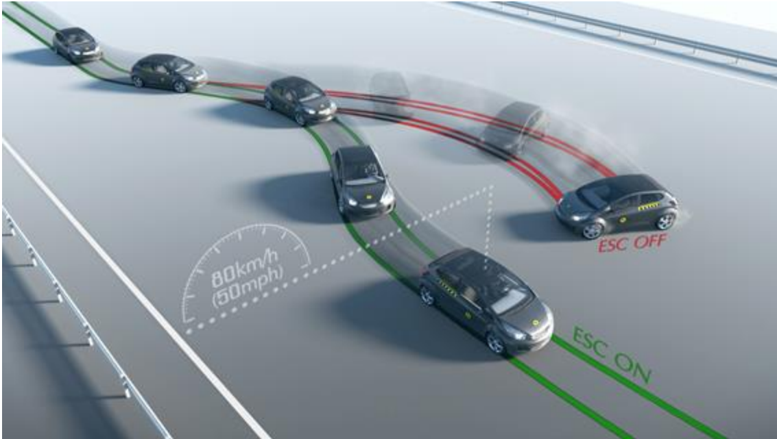
Slika 60. Predodžba ispitivanja ESC-a, izvor: www.euroncap.com/en/vehicle-safety/the-ratings-explained/safety-assist/previous-tests/esc/ [51]
