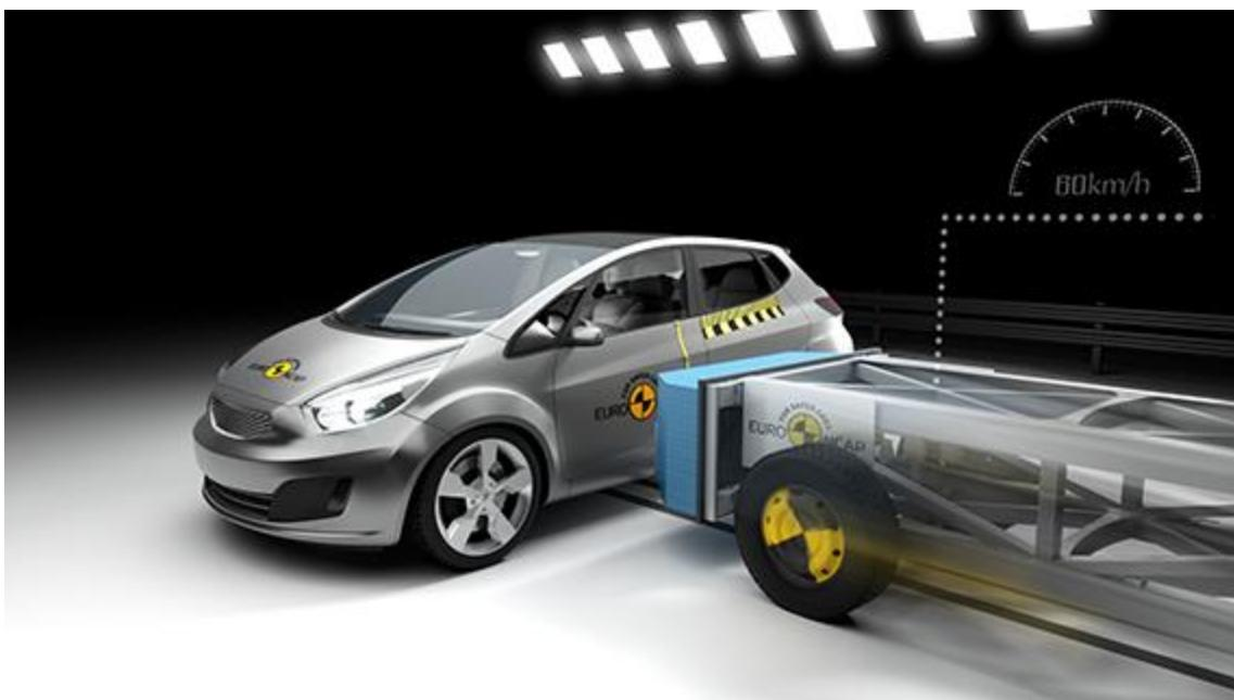
Slika 25. Predodžba SMB testiranja, izvor: [www.euroncap.com/en/vehicle-safety/the-ratings-explained/adult-occupant-protection/lateral-impact/side-mobile-barrier/](http://www.euroncap.com/en/vehicle-safety/the-ratings-explained/adult-occupant-protection/lateral-impact/side-mobile-barrier/) [29]
