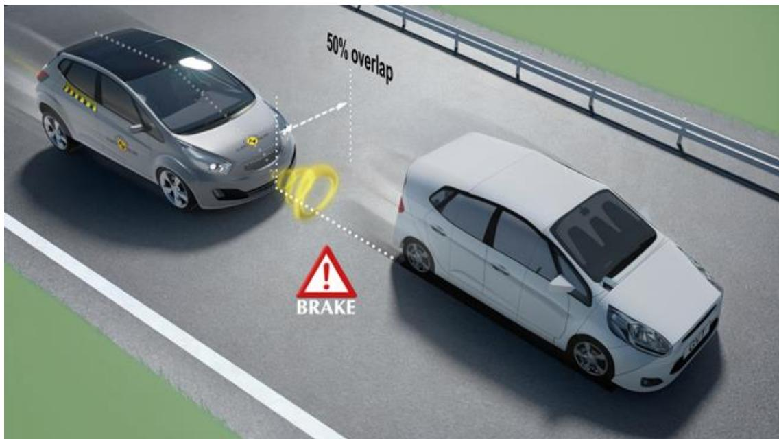
Slika 49. Ispitivanje i izbjegavanje naleta na zaustavljenovo vozilo pomoću AEB sustava, izvor: [www.euroncap.com/en/vehicle-safety/the-ratings-explained/safety-assist/aeb-car-to-car/](http://www.euroncap.com/en/vehicle-safety/the-ratings-explained/safety-assist/aeb-car-to-car/) [45]
