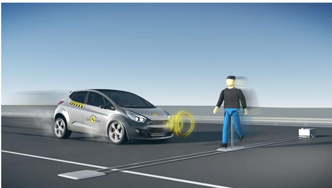
Slika 42. Ispitivanja izbjegavanja naleta vozila prilikom prelaska pješaka preko ceste, izvor: [www.euroncap.com/en/vehicle-safety/the-ratings-explained/vulnerable-road-user-vru-protection/aeb-pedestrian/](http://www.euroncap.com/en/vehicle-safety/the-ratings-explained/vulnerable-road-user-vru-protection/aeb-pedestrian/) [43]
