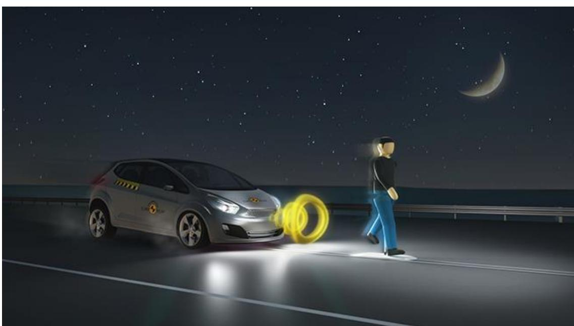
Slika 43. Ispitivanje izbjegavanja pješaka u uvjetima smanjene vidljivosti, izvor: [www.euroncap.com/en/vehicle-safety/the-ratings-explained/vulnerable-road-user-vru-protection/aeb-pedestrian/](http://www.euroncap.com/en/vehicle-safety/the-ratings-explained/vulnerable-road-user-vru-protection/aeb-pedestrian/) [43]
