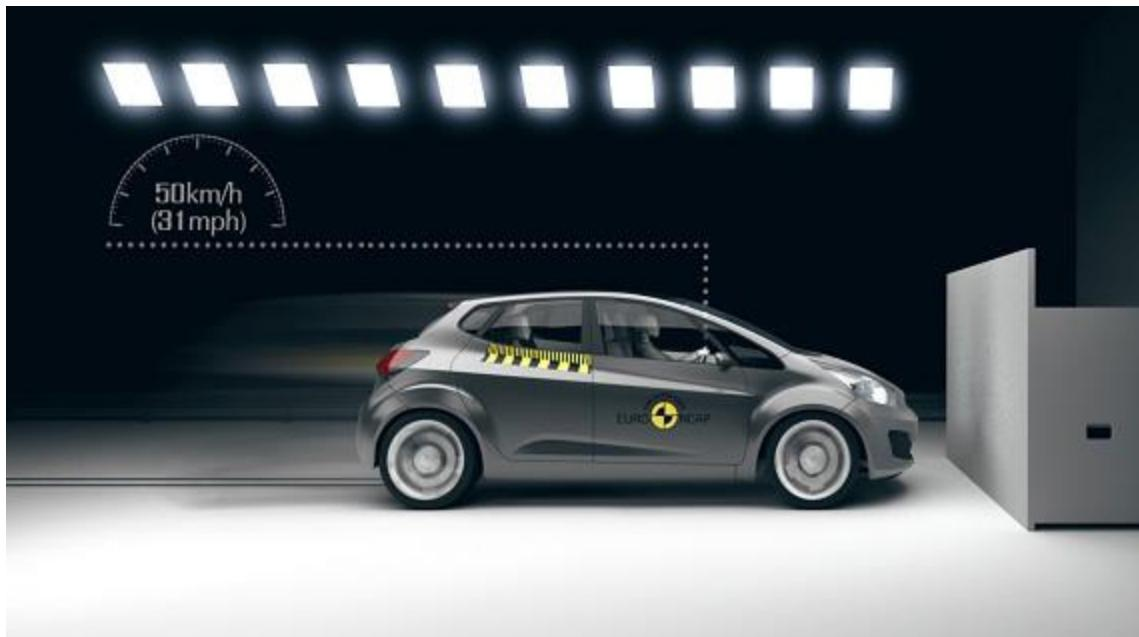
Slika 24. Predodžba FWRB testiranja, izvor: [www.euroncap.com/en/vehicle-safety/the-ratings-explained/adult-occupant-protection/frontal-impact/full-width-rigid-barrier/\[28\]](http://www.euroncap.com/en/vehicle-safety/the-ratings-explained/adult-occupant-protection/frontal-impact/full-width-rigid-barrier/[28])
