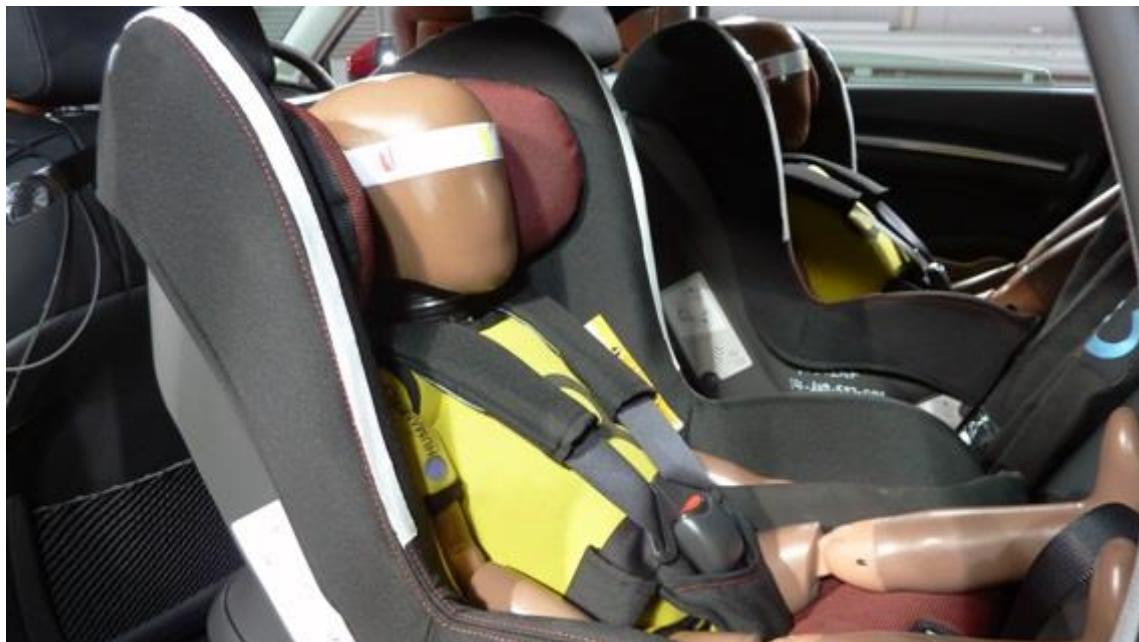
Slika 33. Predodžba CRS ispitivanja, izvor: [www.euroncap.com/en/vehicle-safety/the-ratings-explained/child-occupant-protection/crs-installation-check/](http://www.euroncap.com/en/vehicle-safety/the-ratings-explained/child-occupant-protection/crs-installation-check/) [37]
