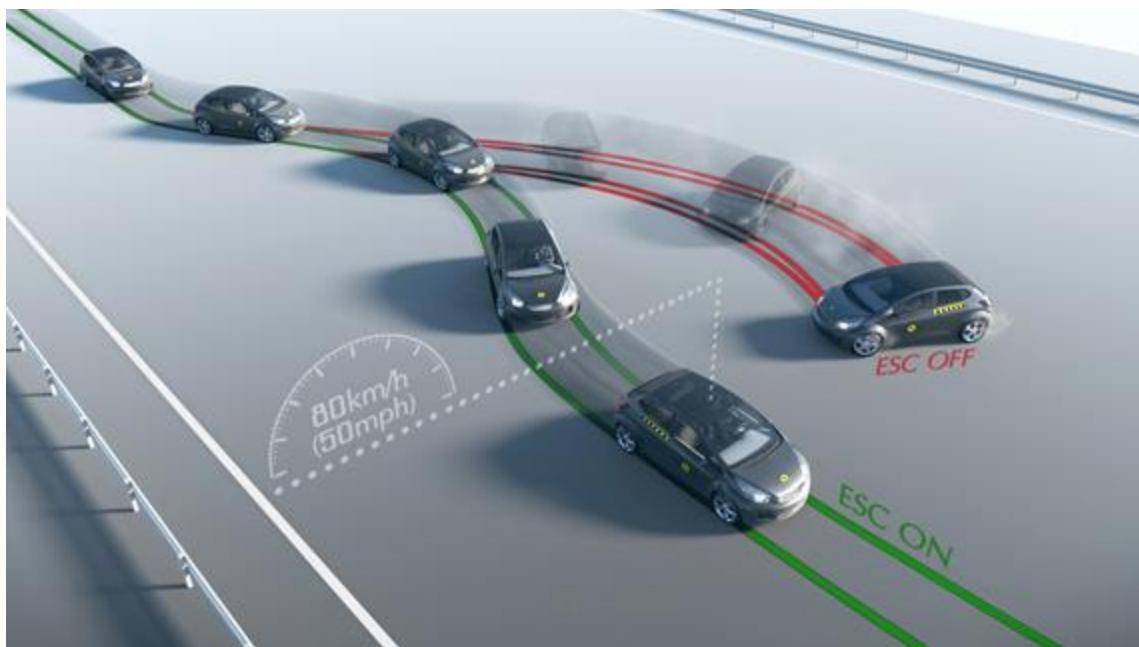
Slika 60. Predodžba ispitivanja ESC-a, izvor: [www.euroncap.com/en/vehicle-safety/the-ratings-explained/safety-assist/previous-tests/esc/](http://www.euroncap.com/en/vehicle-safety/the-ratings-explained/safety-assist/previous-tests/esc/) [51]
