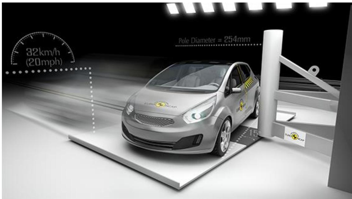
Slika 26. Predodžba SP testiranja, izvor: [www.euroncap.com/en/vehicle-safety/the-ratings-explained/adult-occupant-protection/lateral-impact/side-pole/](http://www.euroncap.com/en/vehicle-safety/the-ratings-explained/adult-occupant-protection/lateral-impact/side-pole/) [30]
