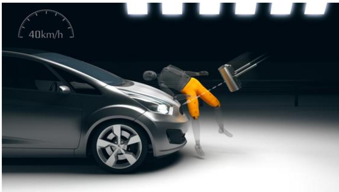
Slika 38. Predodžba Simulacija naleta vozila na gornji dio nogu pješaka, izvor: [www.euroncap.com/en/vehicle-safety/the-ratings-explained/vulnerable-road-user-vru-protection/upper-leg-impact/](http://www.euroncap.com/en/vehicle-safety/the-ratings-explained/vulnerable-road-user-vru-protection/upper-leg-impact/) [41]
