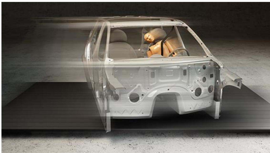
Slika 27. Predodžba FSI testiranja, izvor: [www.euroncap.com/en/vehicle-safety/the-ratings-explained/adult-occupant-protection/lateral-impact/far-side-impact/](http://www.euroncap.com/en/vehicle-safety/the-ratings-explained/adult-occupant-protection/lateral-impact/far-side-impact/) [31]
