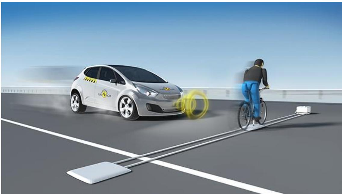
Slika 46. Izbjegavanje naleta vozila na biciklista koji vozi preko putanje vozila, izvor: [www.euroncap.com/en/vehicle-safety/the-ratings-explained/vulnerable-road-user-vru-protection/aeb-cyclist/](http://www.euroncap.com/en/vehicle-safety/the-ratings-explained/vulnerable-road-user-vru-protection/aeb-cyclist/) [44]
