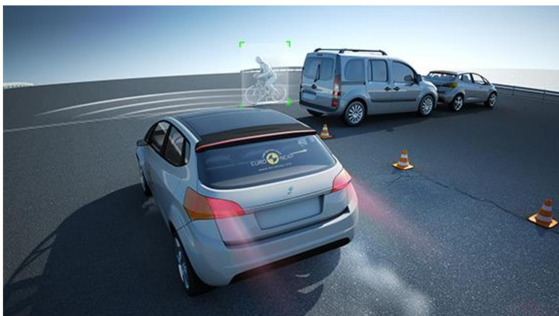
Slika 45. Predodžba ispitivanje izbjegavanja naleta vozila na biciklista zaklonjenog parkiranim vozilima, izvor: [www.euroncap.com/en/vehicle-safety/the-ratings-explained/vulnerable-road-user-vru-protection/aeb-cyclist/](http://www.euroncap.com/en/vehicle-safety/the-ratings-explained/vulnerable-road-user-vru-protection/aeb-cyclist/) [44]
