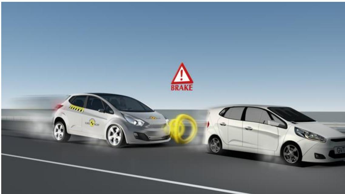
Slika 48. Predodžba ispitivanja zaustavljanja i izbjegavanja naleta na sporije vozilo pomoću AEB sustava, izvor: [www.euroncap.com/en/vehicle-safety/the-ratings-explained/safety-assist/aeb-car-to-car/](http://www.euroncap.com/en/vehicle-safety/the-ratings-explained/safety-assist/aeb-car-to-car/) [45]
