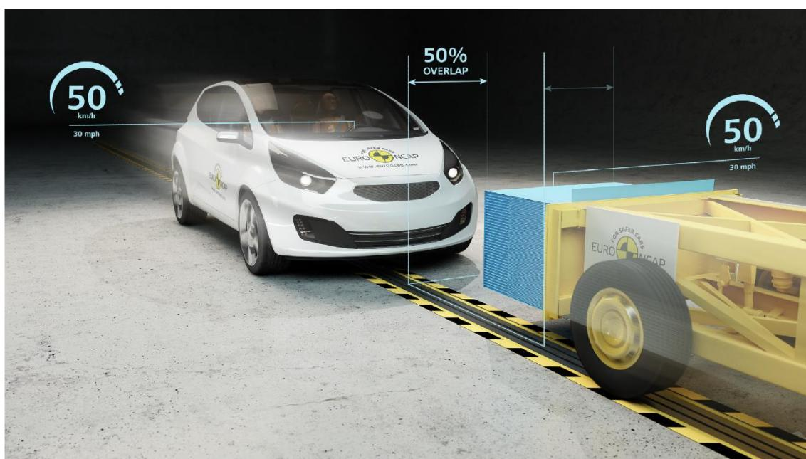
Slika 22. Predodžba MPDB testiranja, izvor: [www.euroncap.com/en/vehicle-safety/the-ratings-explained/adult-occupant-protection/frontal-impact/mobile-progressive-deformable-barrier/](http://www.euroncap.com/en/vehicle-safety/the-ratings-explained/adult-occupant-protection/frontal-impact/mobile-progressive-deformable-barrier/) [25]
