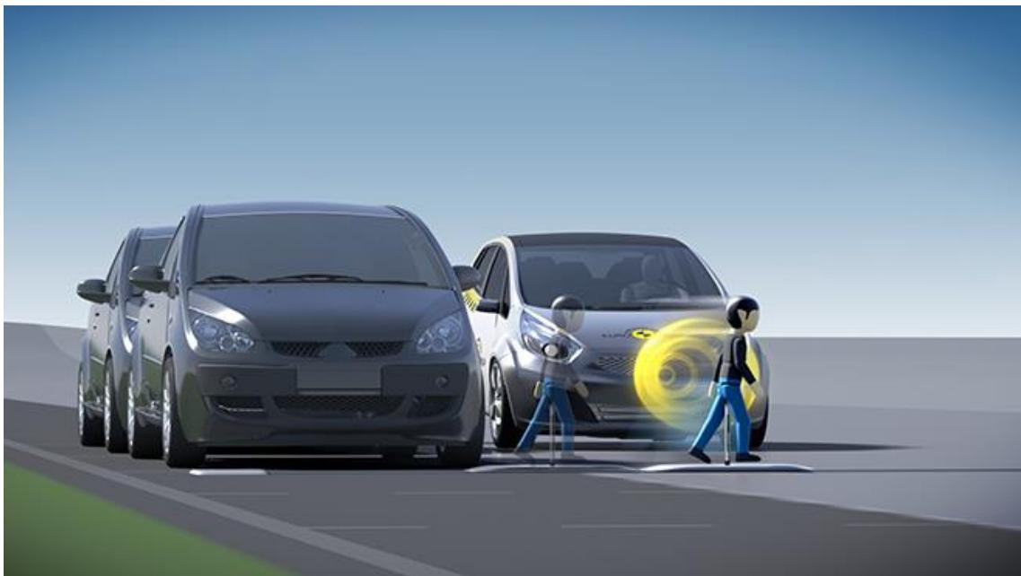
Slika 44. Ispitivanje izbjegavanja naleta vozila na djecu prilikom iznenadnog prelaska ceste iza parkiranog vozila, izvor: [www.euroncap.com/en/vehicle-safety/the-ratings-explained/vulnerable-road-user-vru-protection/aeb-pedestrian/](http://www.euroncap.com/en/vehicle-safety/the-ratings-explained/vulnerable-road-user-vru-protection/aeb-pedestrian/) [43]
