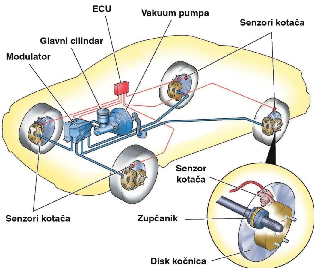
Slika 2. Predodžba načina rada ABS-a, izvor: [www.motor-works.com/blog/inside-the-tech--anti-lock-braking-system--abs \[4\]](http://www.motor-works.com/blog/inside-the-tech--anti-lock-braking-system--abs)
