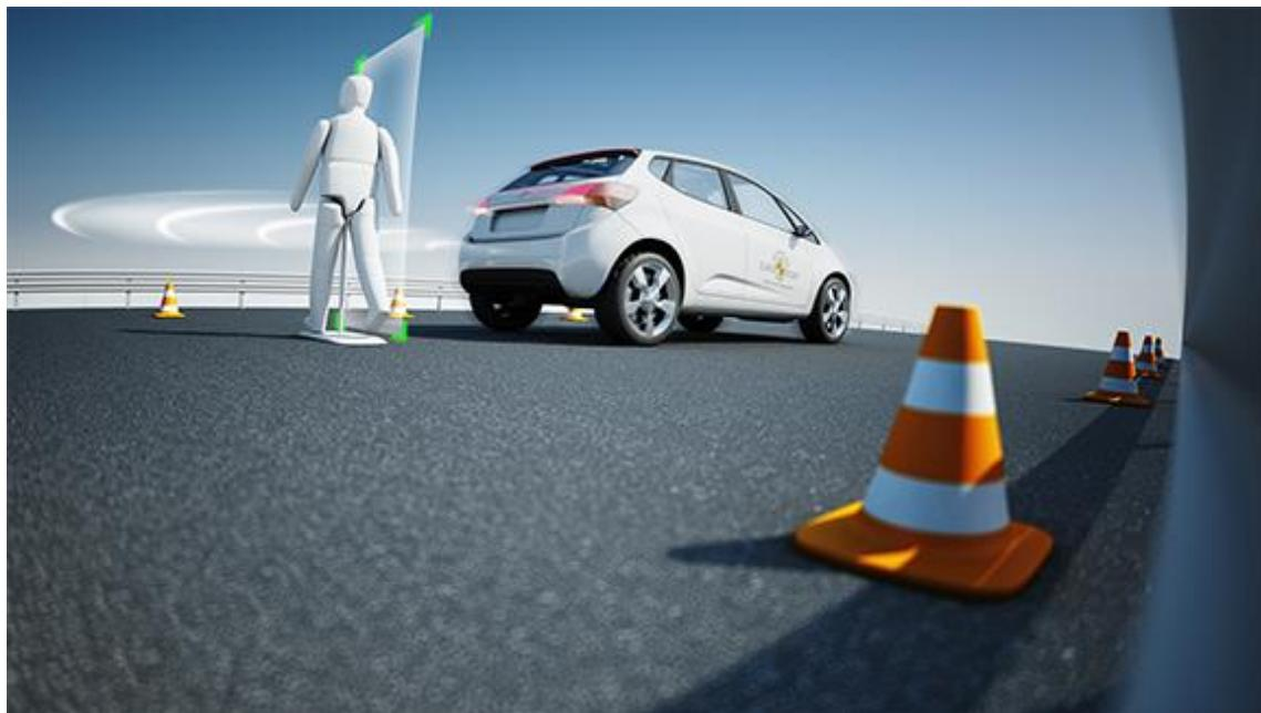
Slika 40. Ispitivanja izbjegavanja naleta na pješaka prilikom vožnje u nazad, izvor: [www.euroncap.com/en/vehicle-safety/the-ratings-explained/vulnerable-road-user-vru-protection/aeb-pedestrian/](http://www.euroncap.com/en/vehicle-safety/the-ratings-explained/vulnerable-road-user-vru-protection/aeb-pedestrian/) [43]
