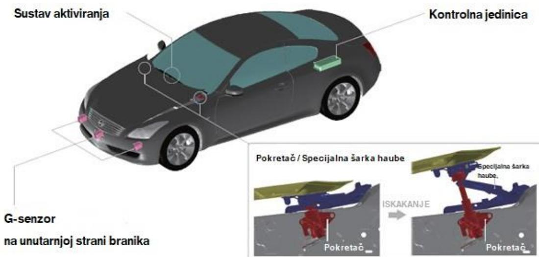
Slika 35. Predodžba osnovnih dijelova pop-up haube, Mazda, izvor: [www.nissan-global.com/EN/TECHNOLOGY/OVERVIEW/puehfpp.html](http://www.nissan-global.com/EN/TECHNOLOGY/OVERVIEW/puehfpp.html) [39]
