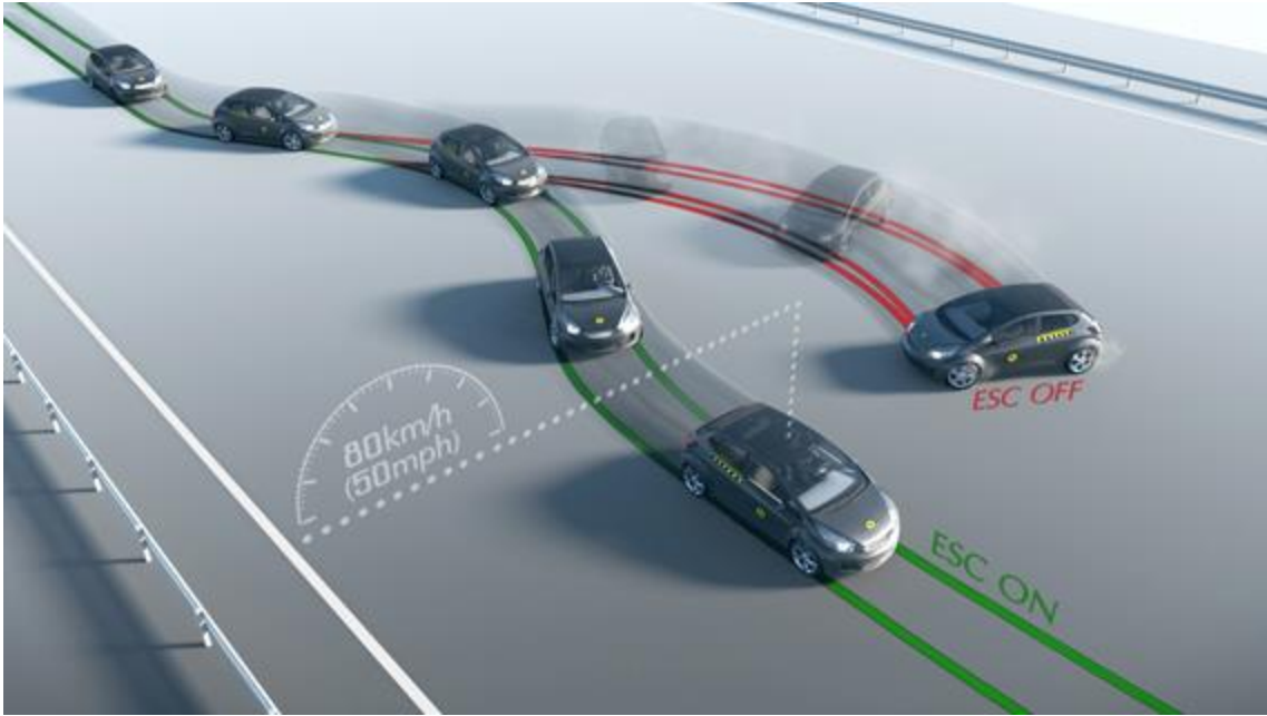
Slika 60. Predodžba ispitivanja ESC-a, izvor: www.euroncap.com/en/vehicle-safety/the-ratings-explained/safety-assist/previous-tests/esc/ [51]
