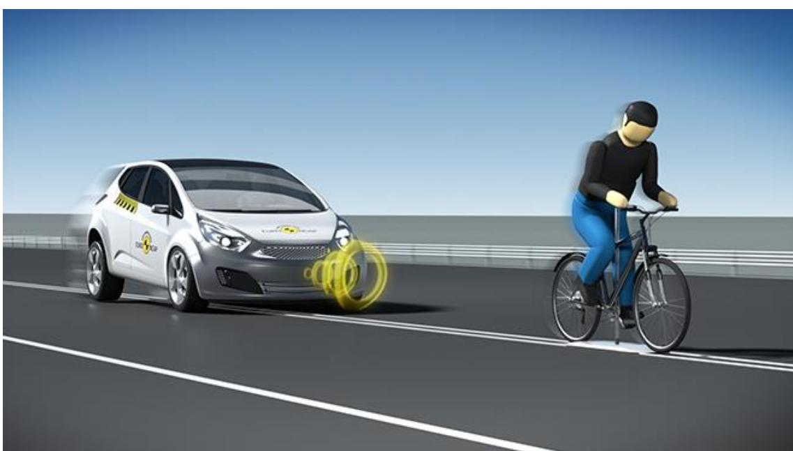
Slika 47. Izbjegavanje naleta vozila na biciklista koji vozi putanjom vozila, izvor: [www.euroncap.com/en/vehicle-safety/the-ratings-explained/vulnerable-road-user-vru-protection/aeb-cyclist/](http://www.euroncap.com/en/vehicle-safety/the-ratings-explained/vulnerable-road-user-vru-protection/aeb-cyclist/) [44]
