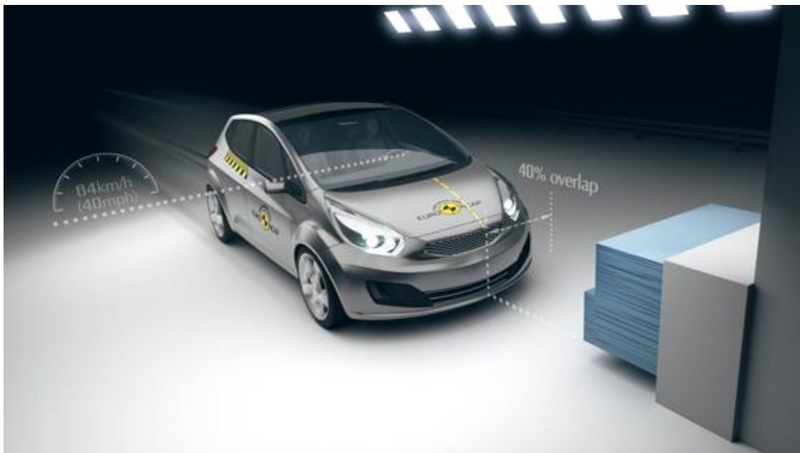
Slika 23. Predodžba ODB testiranja, izvor: www.euroncap.com/en/vehicle-safety/the-ratings-explained/adult-occupant-protection/previous-tests/offset-deformable-barrier [27]
