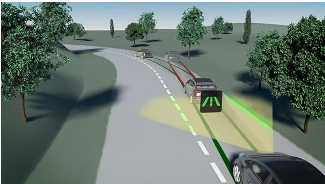
Slika 59. Prikaz održavanja vozne trake i prepoznavanja ruba ceste, izvor: [www.euroncap.com/en/vehicle-safety/the-ratings-explained/safety-assist/lane-support/](http://www.euroncap.com/en/vehicle-safety/the-ratings-explained/safety-assist/lane-support/) [48]
