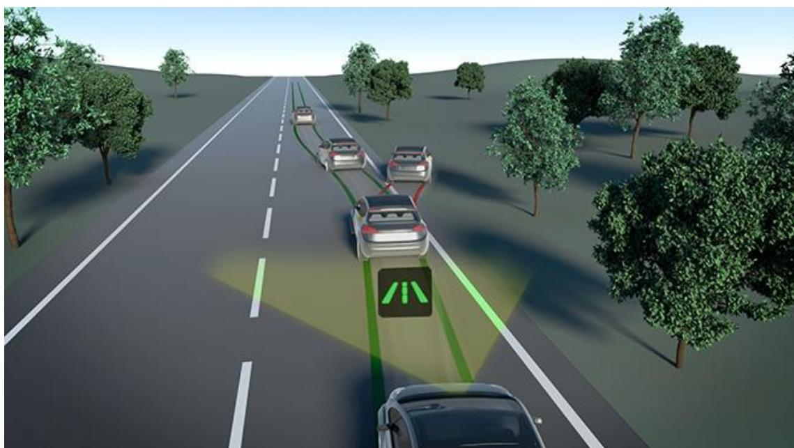
Slika 58. Prikaz održavanja vozne trake, izvor: [www.euroncap.com/en/vehicle-safety/the-ratings-explained/safety-assist/lane-support/](http://www.euroncap.com/en/vehicle-safety/the-ratings-explained/safety-assist/lane-support/) [48]
