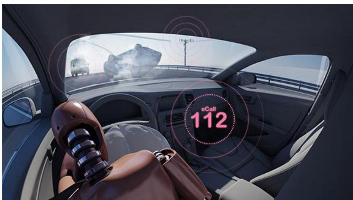
Slika 29. Predodžba eCall sustava, izvor: [www.euroncap.com/en/vehicle-safety/the-ratings-explained/adult-occupant-protection/rescue-and-extrication/](http://www.euroncap.com/en/vehicle-safety/the-ratings-explained/adult-occupant-protection/rescue-and-extrication/) [33]
