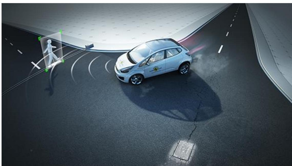
Slika 41. Ispitivanje izbjegavanje naleta na pješaka prilikom skretanja vozila, izvor: [www.euroncap.com/en/vehicle-safety/the-ratings-explained/vulnerable-road-user-vru-protection/aeb-pedestrian/](http://www.euroncap.com/en/vehicle-safety/the-ratings-explained/vulnerable-road-user-vru-protection/aeb-pedestrian/) [43]
