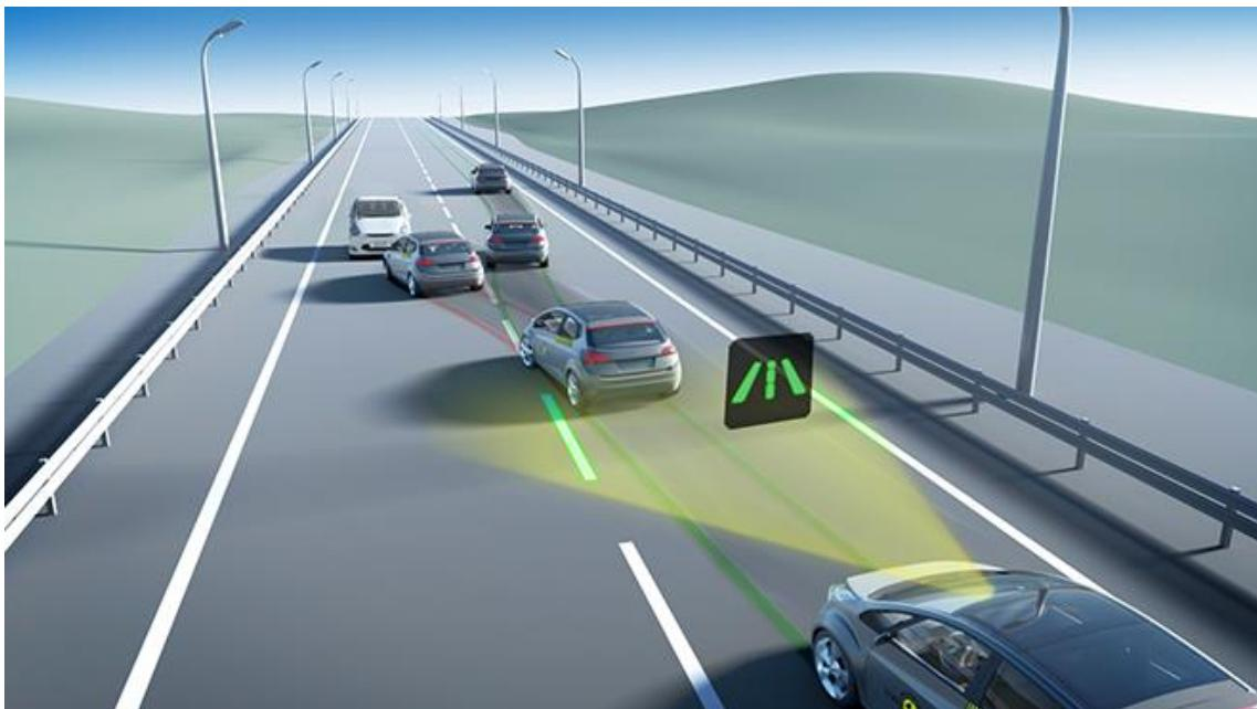
Slika 54. Prikaz aktiviranja ELK sustava na nadolazeći promet i vraćanja vozila u svoju traku, izvor: [www.euroncap.com/en/vehicle-safety/the-ratings-explained/safety-assist/lane-support/](http://www.euroncap.com/en/vehicle-safety/the-ratings-explained/safety-assist/lane-support/) [48]
