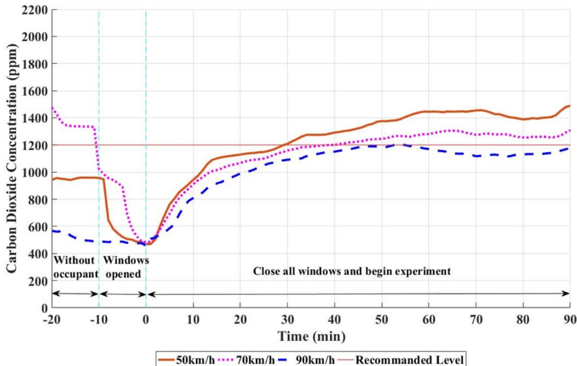
Slika 9. Predodžba razine (ppm) ugljičnog dioksida u vozilu sa jednim putnikom, izvor: [www.researchgate.net/figure/The-carbon-dioxide-concentration-and-increase-the-vehicle-speed-against-time-with-two\\_fig4\\_312194065 \[14\]](http://www.researchgate.net/figure/The-carbon-dioxide-concentration-and-increase-the-vehicle-speed-against-time-with-two_fig4_312194065)
