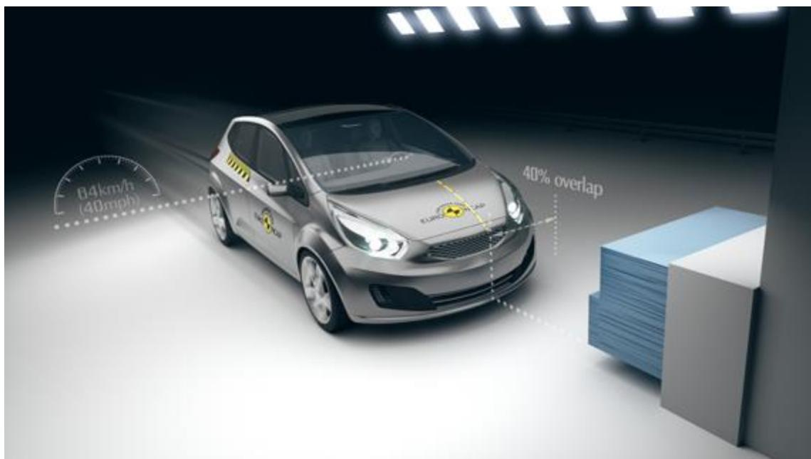
Slika 23. Predodžba ODB testiranja, izvor: [www.euroncap.com/en/vehicle-safety/the-ratings-explained/adult-occupant-protection/previous-tests/offset-deformable-barrier](http://www.euroncap.com/en/vehicle-safety/the-ratings-explained/adult-occupant-protection/previous-tests/offset-deformable-barrier) [27]
