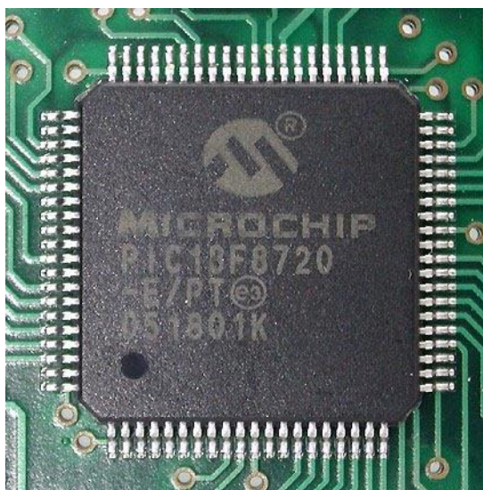
Slika 4. 80 pin-ski microcontroller. [Izvor: https://en.wikipedia.org/wiki/Microcontroller ]
