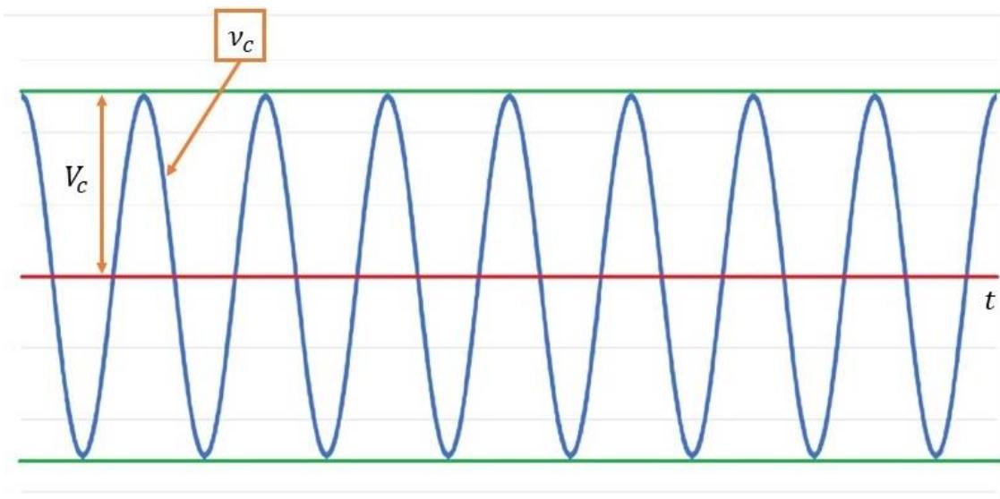
Slika 6. Prikaz signala nosioca (carrier)
