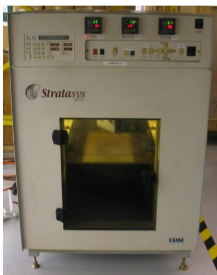
Slika 19. Stratasys FDM 1600 printer. [19]
