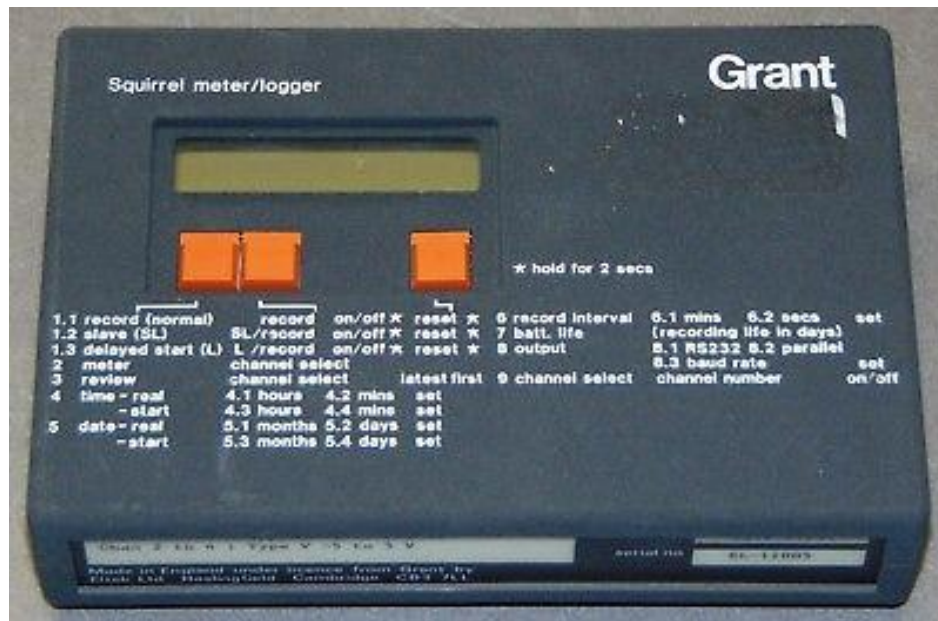
Slika 12 Grant Squirrel meter/logger ( www.ebay.com )
