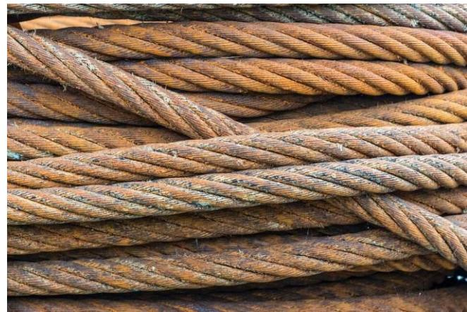
Slika 10: Korozirano čelično uže (<https://www.wire-rope-direct.com/wp-content/uploads/2016/10/Corroded-Wire-Rope.jpg>)
