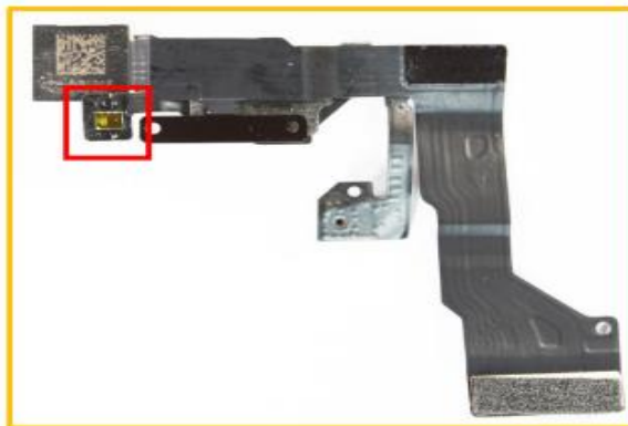
light sensor (mnf. unknown) 1.85 mm x 1.30 mm x 0.50 mm
