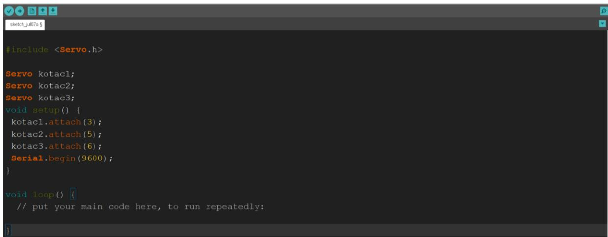
The screenshot shows the Arduino IDE interface with a sketch titled "sketch\_jul07a". The code defines three servos: kotac1, kotac2, and kotac3. In the setup() function, each servo is attached to pins 3, 5, and 6 respectively. The Serial.begin(9600) command initializes the serial port at 9600 baud. The loop() function is empty, indicated by a single brace {}, with a note: // put your main code here, to run repeatedly:.
