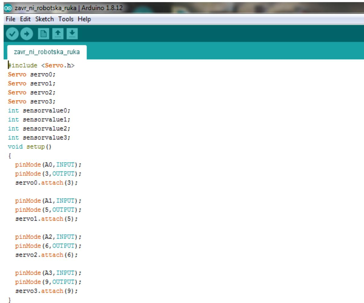
The screenshot shows the Arduino IDE interface with the title bar "zavr\_ni\_robotska\_ruka | Arduino 1.8.12". The menu bar includes File, Edit, Sketch, Tools, and Help. Below the menu is a toolbar with icons for save, upload, and other functions. The main area displays the following C++ code:
