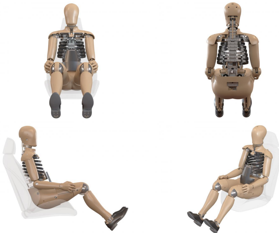
Slika 21. Predodžba modela THOR-50M, izvor: humanetics.humaneticsgroup.com/products/anthropomorphic-test-devices/frontal-impact/thor-50m/thor-50m [26]
