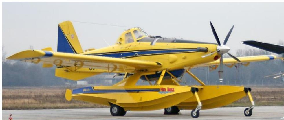
Slika 7. Zrakoplov Air Tractor 802 A (Fire Boss) [12]
