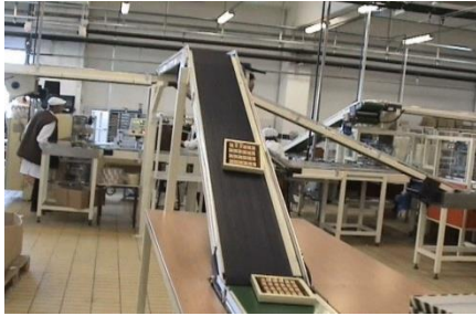
Slika 2. Transportna traka ( http://www.kopack.hr/ )
