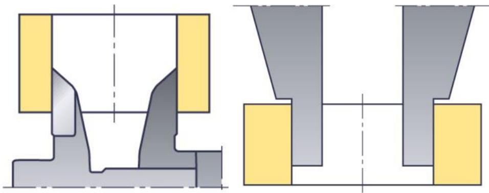
**Slika 9.** Unutarnje mjerjenje
