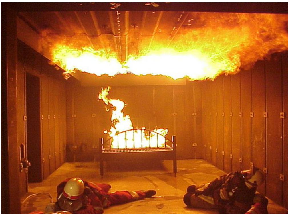
Sl. 13. Obuka vatrogasaca na flashover simulatoru [14]
