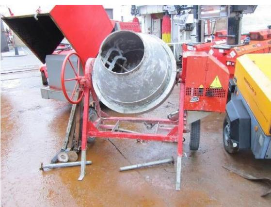
Slika 13 Prikaz betonske mješalice [[https://autoline.hr/img/s/gradevinska-oprema-betonska-mjesalicaMANITOU-BF-BSI-340-S---1\\_big--13120515321757706200.jpg](https://autoline.hr/img/s/gradevinska-oprema-betonska-mjesalicaMANITOU-BF-BSI-340-S---1_big--13120515321757706200.jpg)]
