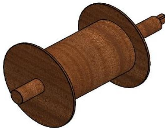
**SLIKA 31.** 3D model bubenja s osovinom
