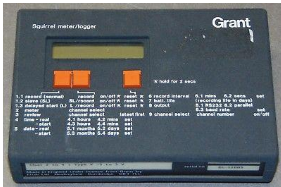
Slika 12 Grant Squirrel meter/logger ( www.ebay.com )
