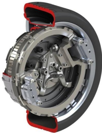
Slika 14. Protean In-wheel motor
