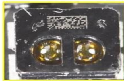
proximity sensor (mnf. unknown) 2.78 mm x 2.38 mm x 1.28 mm
