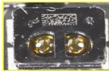
proximity sensor (mnf. unknown) 2.78 mm x 2.38 mm x 1.28 mm
