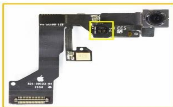
proximity sensor (mnf. unknown) 2.78 mm x 2.38 mm x 1.28 mm
