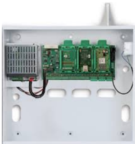
Slika 04. Predodžba Protuprovalna centrala. Izvor: https://encrypted-tbn0.gstatic.com/images?q=tbn:ANd9GcQfc5SyAwaLog6teIAITrUXDj8WPcphMmWBYRWeMkJ1u2y2OUoS0w
