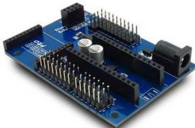
Slika 27: Arduino Nano IO shield [27]
