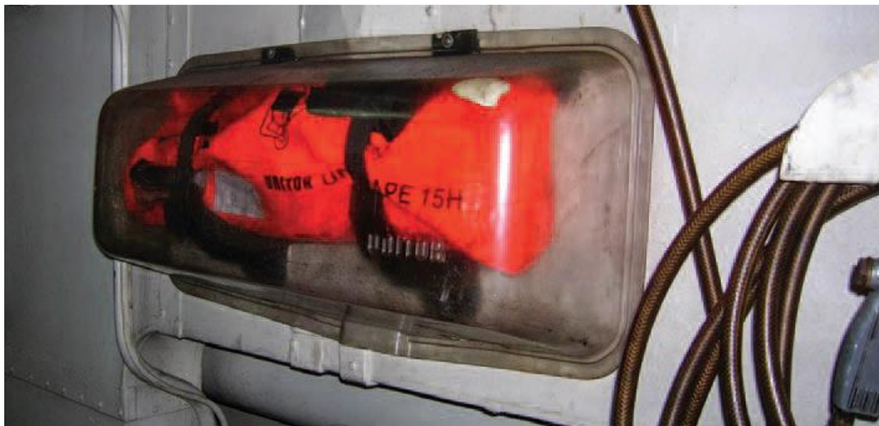
Slika 10. EEBD ( Emergency Escape Breathing Device)
