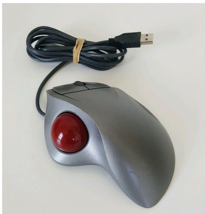
Slika 27: Logitech Trackball Mouse T-BB18 [7]
