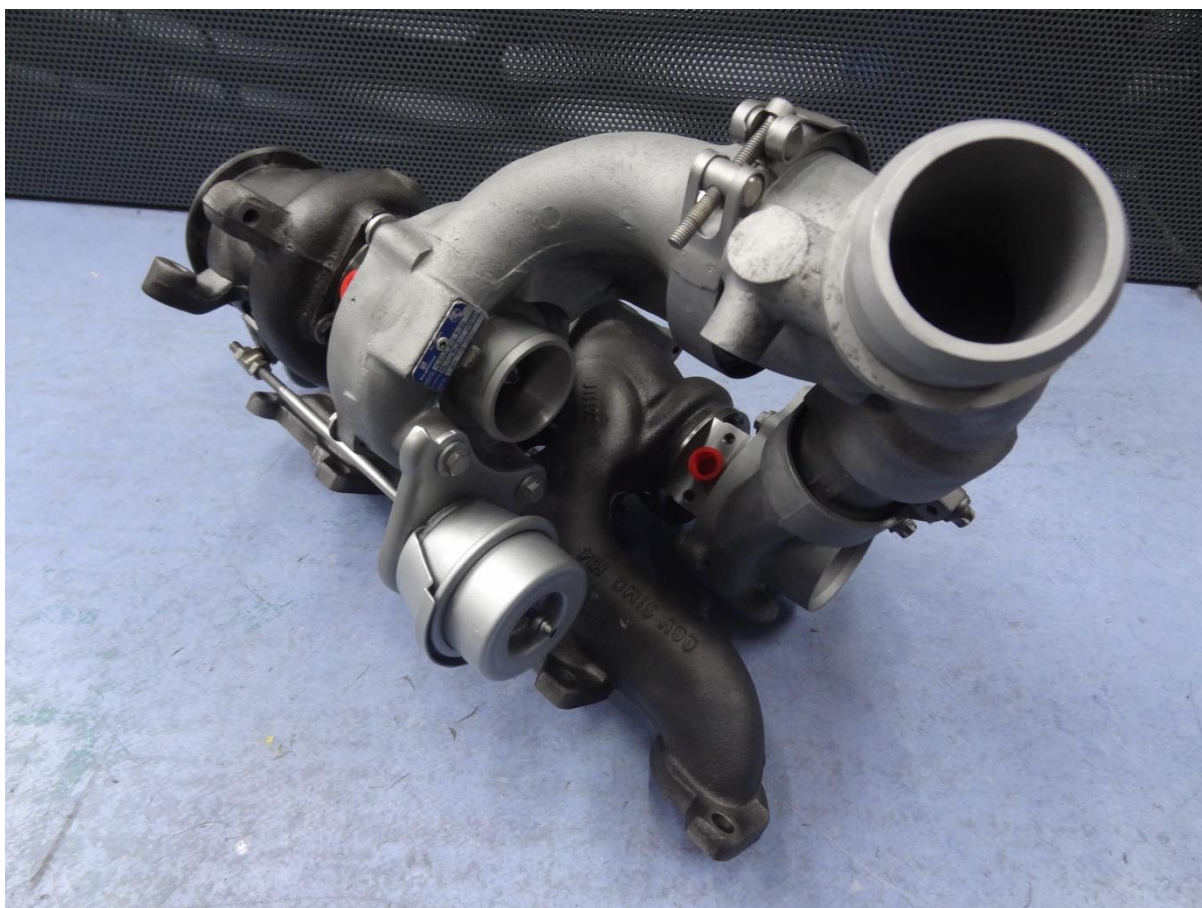
Slika 34 Borgwarner BI-turbopunjač, MB Sprinter 215 CDI [17]
