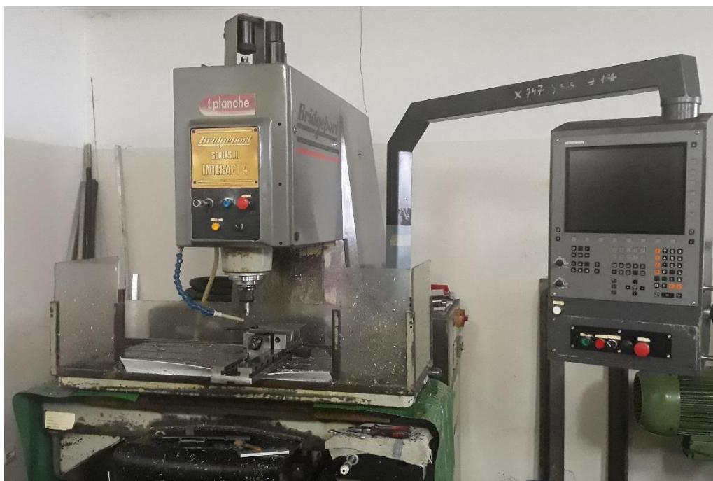
Slika 45. CNC glodalica Bridgeport Interact 4
