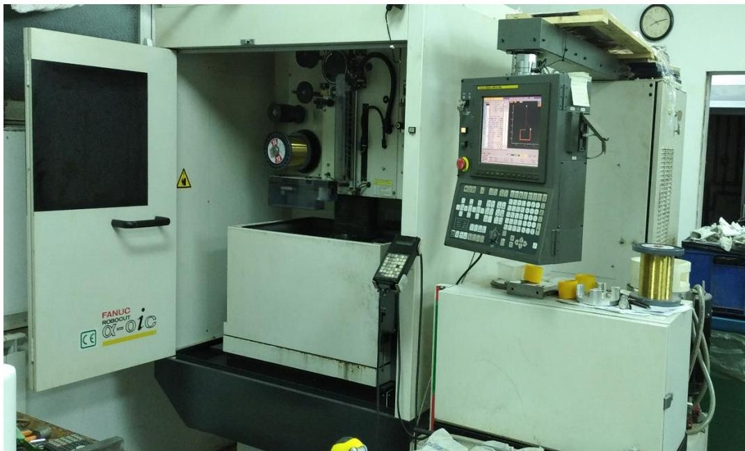
Slika 51. EDM Fanuc RoboCut
