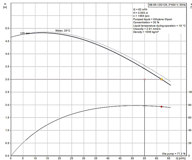
Slika 6.22. Dijagram radne točke pumpe Grundfos NB 65-125/125 A-F2-A-E-BQQE [12]
