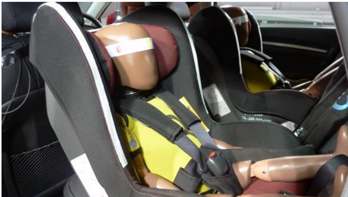
Slika 33. Predodžba CRS ispitivanja, izvor: www.euroncap.com/en/vehicle-safety/the-ratings-explained/child-occupant-protection/crs-installation-check/ [37]
