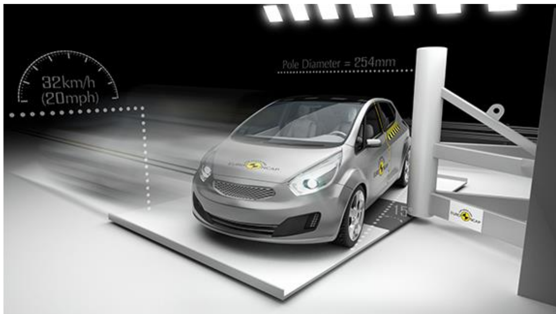
Slika 26. Predodžba SP testiranja, izvor: www.euroncap.com/en/vehicle-safety/the-ratings-explained/adult-occupant-protection/lateral-impact/side-pole/ [30]
