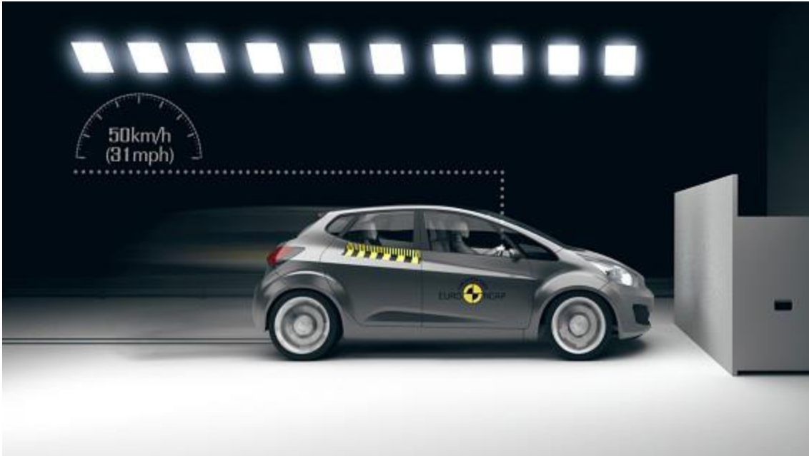
Slika 24. Predodžba FWRB testiranja, izvor: www.euroncap.com/en/vehicle-safety/the-ratings-explained/adult-occupant-protection/frontal-impact/full-width-rigid-barrier/ [28]
