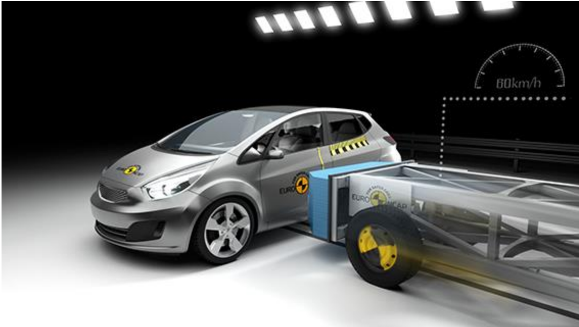
Slika 25. Predodžba SMB testiranja, izvor: www.euroncap.com/en/vehicle-safety/the-ratings-explained/adult-occupant-protection/lateral-impact/side-mobile-barrier/ [29]
