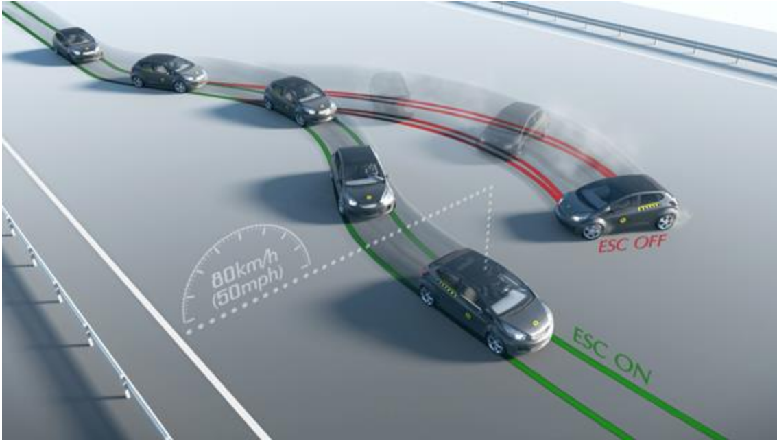
Slika 60. Predodžba ispitivanja ESC-a, izvor: www.euroncap.com/en/vehicle-safety/the-ratings-explained/safety-assist/previous-tests/esc/ [51]
