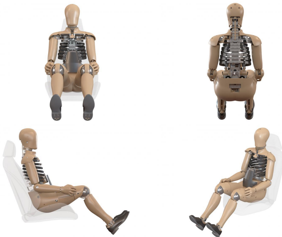
Slika 21. Predodžba modela THOR-50M, izvor: humanetics.humaneticsgroup.com/products/anthropomorphic-test-devices/frontal-impact/thor-50m/thor-50m [26]
