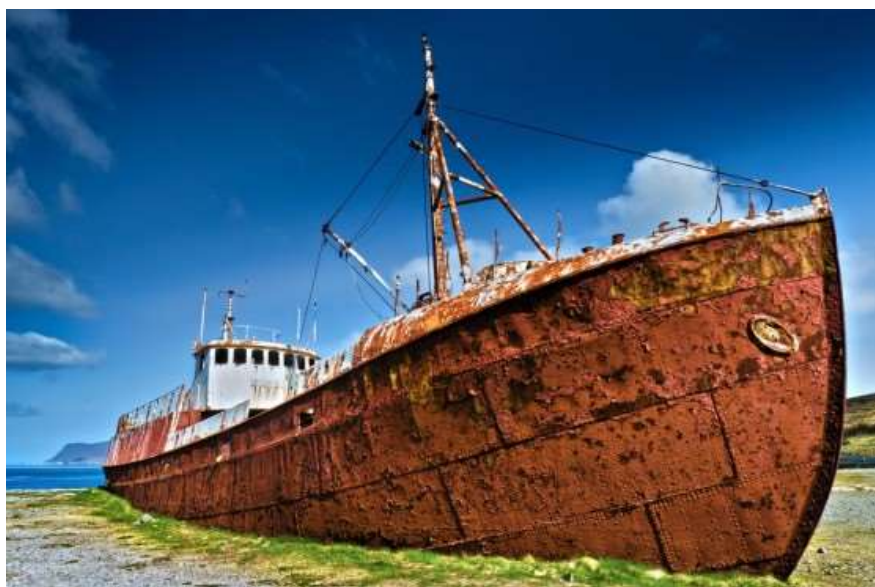
Slika 5. Korozija trupa broda ( https://thenavalarch.com/ship-corrosion-cathodic-protection-sacrificial-anodes/ Pristupljeno 15.07.2021)
