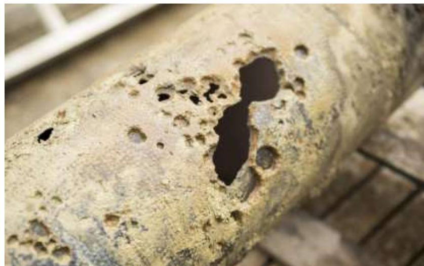
**Slika 9.** Primjer rupičaste(pitting) korozije (<https://www.nuflowmidwest.com/2-types-of-corrosion-that-occur-in-industrial-piping-systems/> Pриступлено 15.07.2021)
