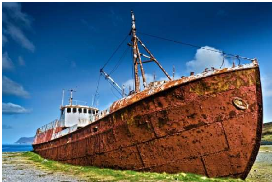
Slika 5. Korozija trupa broda ( https://thenavalarch.com/ship-corrosion-cathodic-protection-sacrificial-anodes/ Pristupljeno 15.07.2021)
