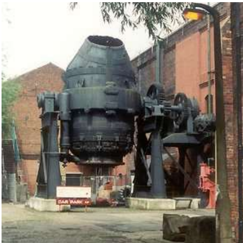
Slika 2. Bessemer i Thomasov postupak ( https://www.britannica.com/technology/Bessemer-process Pristupljeno 02.07.2021.)
