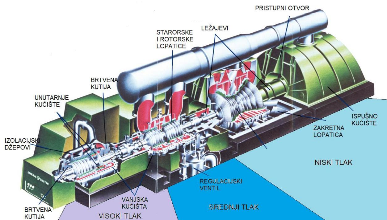
Slika 6. General Electric - parna turbina velike snage [3]
