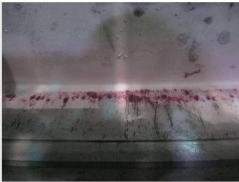
Erosion highlighted by the DPI test
