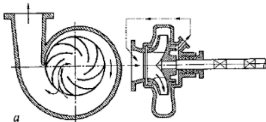
Slika 2. Spiralno kućište centrifugalne pumpe (Izvor: <https://core.ac.uk/>) [11]
