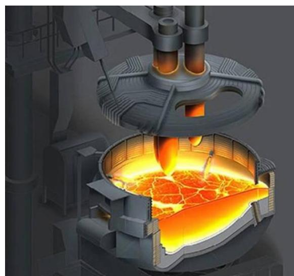
**Slika 2.** Elektrolučna peć (<https://www.exportersindia.com/product-detail/electric-arc-furnace-818224.htm>, Pristupljeno 15.12.2022.)
