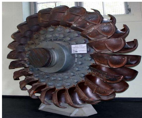
Slika 4. Peltonova turbina [3]
