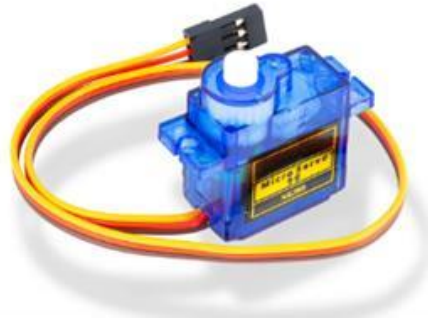
Slika 6: Servo motor TowerPro SG90
