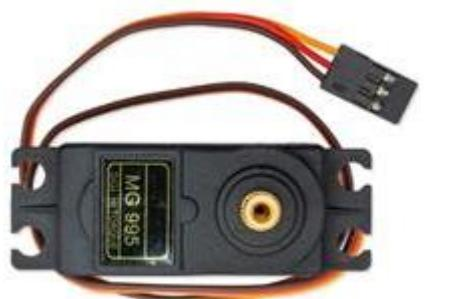
Slika 5: Servo motor TowerPro MG995
