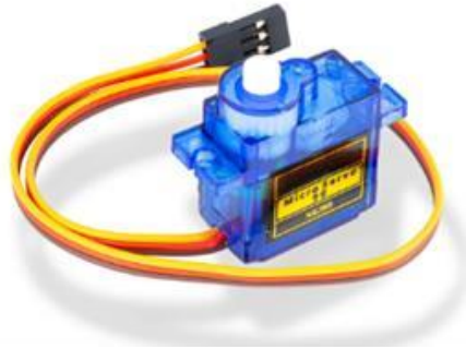
Slika 6: Servo motor TowerPro SG90
