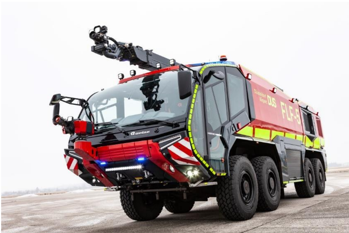
Slika 2. Rosenbauer Panther 8x8, 12500l vode/1500l pjenila/250kg praha
