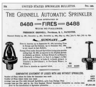
Slika 5. Frederick Grinnell patent sprinkler mlaznice ( https://www.ibs-austria.at/wp-content/uploads/2021/11/2017_IBS_SPR_Infolder.pdf )
