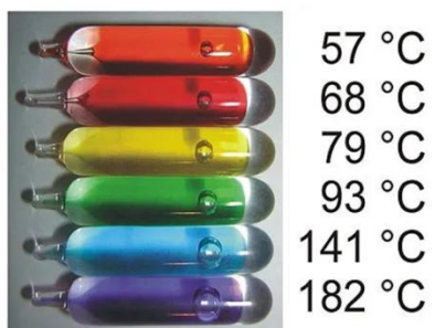
Slika 8. Prikaz staklene ampule, temperatura aktiviranja raspoznaje se po boji ampule https://blog.adafruit.com/2017/11/06/how-a-fire-sprinkler-works-including-color-coding-various-designs/ )
