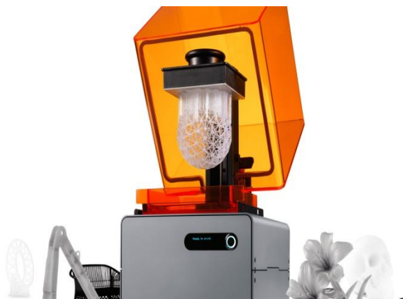
Slika 3. FormLab desktop SLA 3D printer [3]
